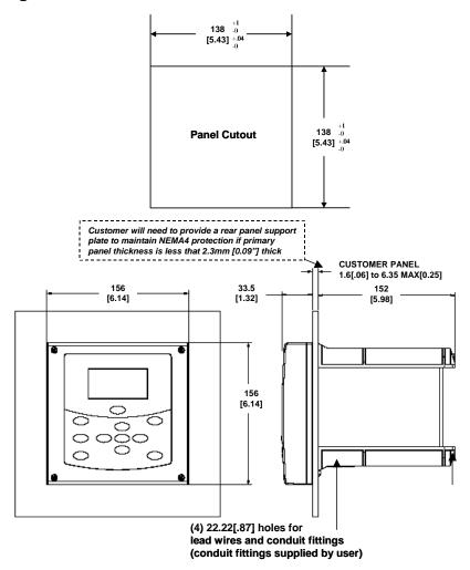
Figure 3-1 Panel Mounting Dimensions (not to scale)
